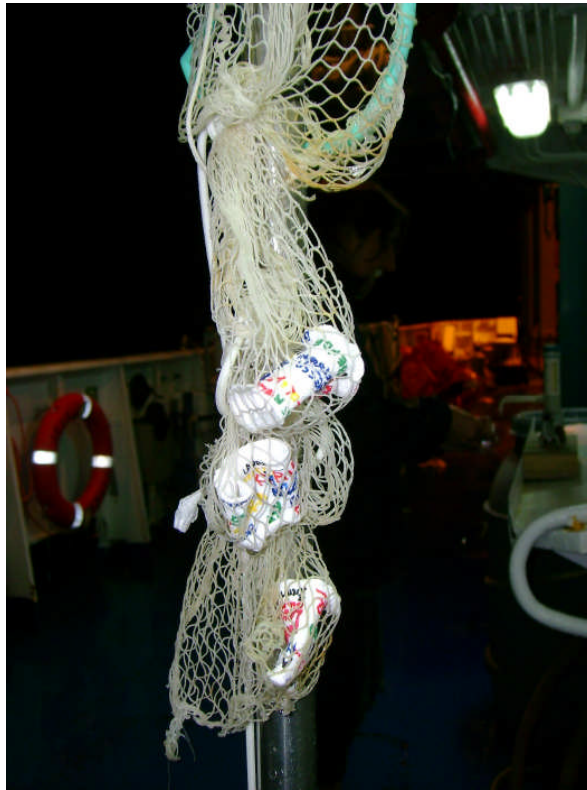
Fig. 10: the cups are recovered after the cast, the effect of pressure is clearly visible
